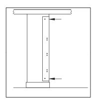
6. Use 1002664 **Button Head** Screws - 3/8" and 1002666 Sex Bolts to secure Alcove Joggle Bracket to 1/2" Thick Panel.
