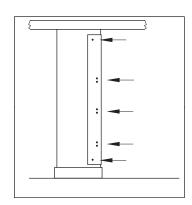
5. Drill 1/4" diameter holes through 1/2" thick panel using hole pattern of Alcove Joggle Brackets (mounted to U-channel on stile) as template.
