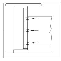
3. Use 1002665 **Button Head** Screws - 5/8" and 1002666 Sex Bolts in topmost and bottom-most holes to secure **U-Channel Bracket** to stile.
