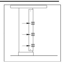
2. Drill 1/4" diameter holes through Solid Color Reinforced Composite (SCRC) material. Use holes on U-Channel as a template.
