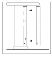
4. Use 1002665 **Button Head** Screws - 5/8" and 1002666 Sex Bolts to attach (3) 1000282 Alcove Joggle Brackets onto 3/4" U-Channel. Place **Alcove Joggle** Brackets on inside of toilet stall.
