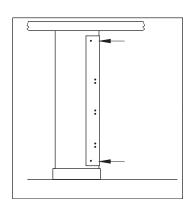
5. Drill 3/16" diameter x 7/16" holes (**Do** not drill thru) on 1/2" thick panel using hole pattern of Alcove Joggle Brackets (mounted to U-channel on stile) as template.
