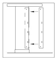
4. Drill 3/16" diameter x 7/16" holes (Do not drill thru). Attach (3) 1000282 Alcove Joggle Brackets onto 3/4" U-Channel using 1002499 Torx Screws. Place Alcove Joggle Brackets on inside of toilet stall.
