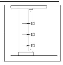
Drill 1/4" diameter holes through Solid Color Reinforced Composite (SCRC) material. Use holes on U-Channel as a template.
