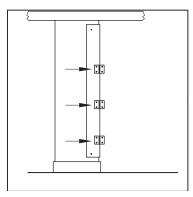
Drill 1/4" diameter holes through Phenolic (top and bottom only). Use holes on U-Channel as a template.
